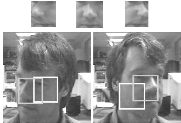
Figure 5: Running example of our tracker. The white rectangle shows where the original template matched, the gray rectangle shows where the rotation template matched. The original and the rotated templates are shown above.
